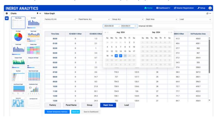
· View data analysis in column format for total energy consumption, easily identify abnormal data over time
