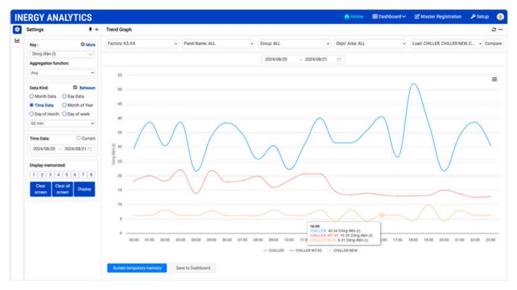
• ·Compare and perform multidimensional analysis between loads, areas, or the same load on different days to identify anomalies in energy usage
